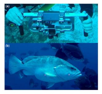
**Figure 2.** Laser caliper system used to measure fish lengths *in situ*. Two parallel laser diodes are placed 20 cm apart inside a custom-machined acrylic housing, with a GoPro Hero<sup>TM</sup> camera in separate housing mounted in front. (a) A diver using the system. (b) Example still-frame image with the two laser dots on a fish perpendicular to the camera. The known distance between the laser dots is used as a scale to measure total length.
